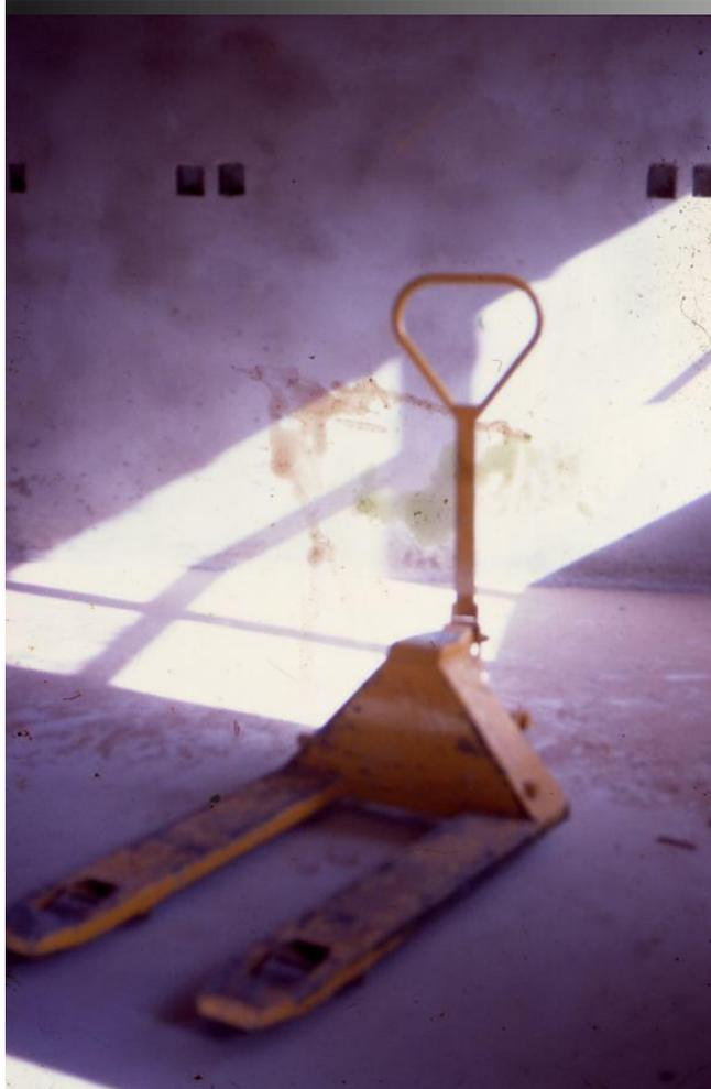
**Pallet trolley used to move pallets of bricks at level of use, Port Elizabeth (Smallwood, 1991)**
